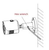
6 Tighten the screws with hex wrench to complete the installation.
