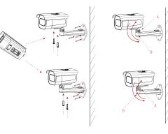
Fix the camera to the bracket with Adjust the viewing angle. screws. The bracket head can be pre-mounted or post-mounted, and then fixed to the wall with 4 screws.
