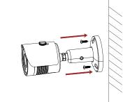
Fix the bracket to the wall with screws.
