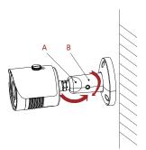
Ø Adjust the viewing angle. Loosen the screws to adjust the angle (A for vertical angle, B for axial angle).
